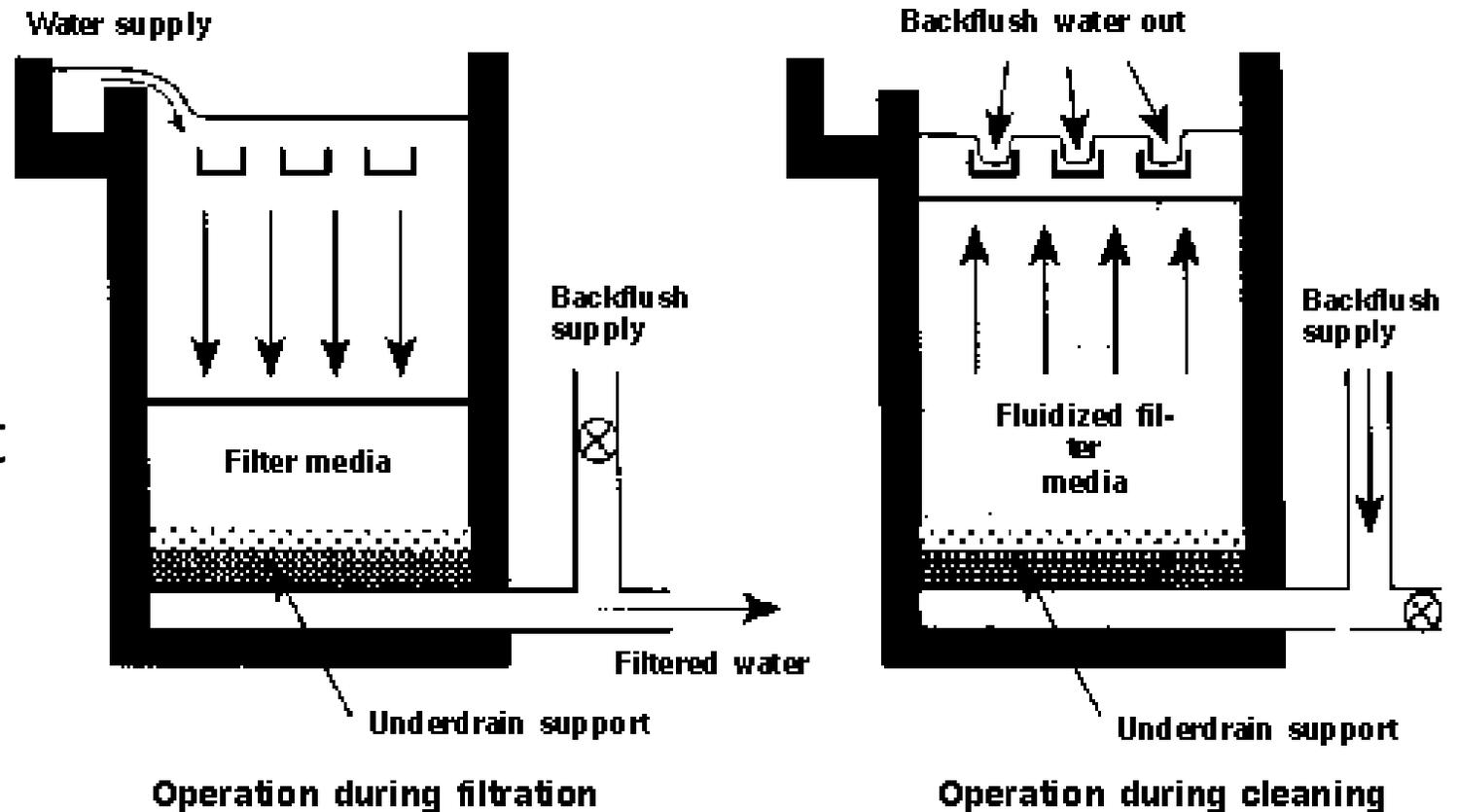
Cross-section of a rapid sand filter.
