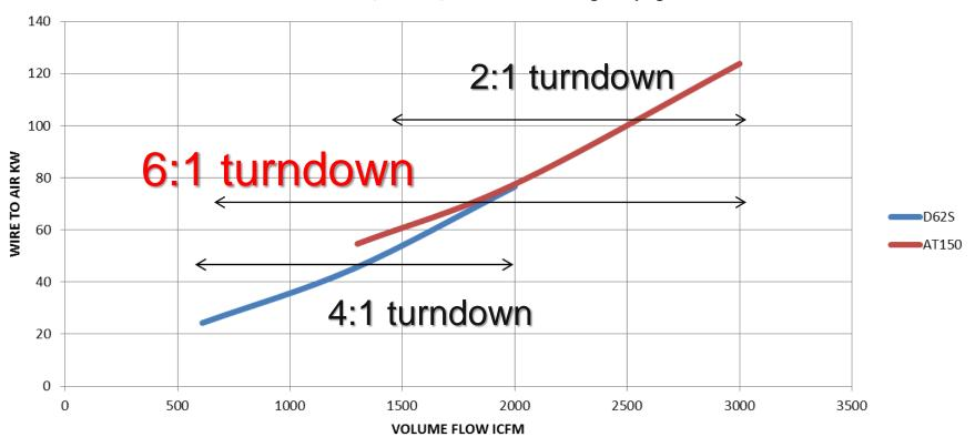
**Turbo plus Hybrid** Inlet: 90 F, 90% RH, 800 fasl ... Discharge: 9 psig
