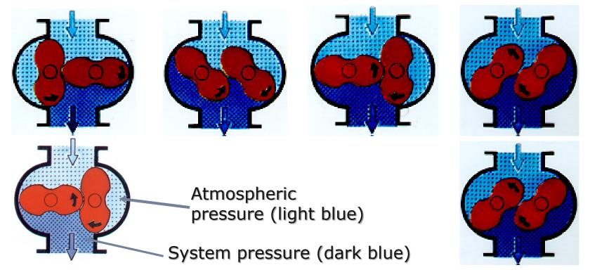
Pressurized air in discharge is about to return into blower housing
