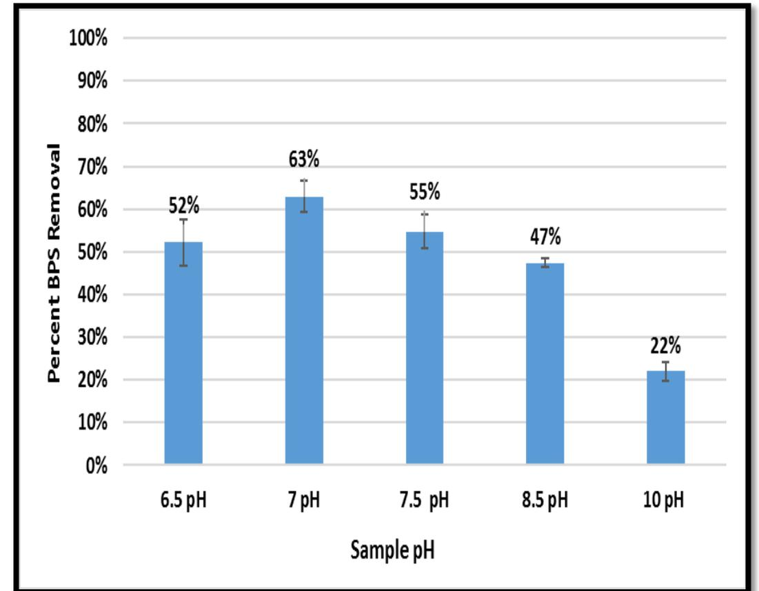
**Optimal removal at pH 7 (315 mg/g; 63% BPS removal)**
