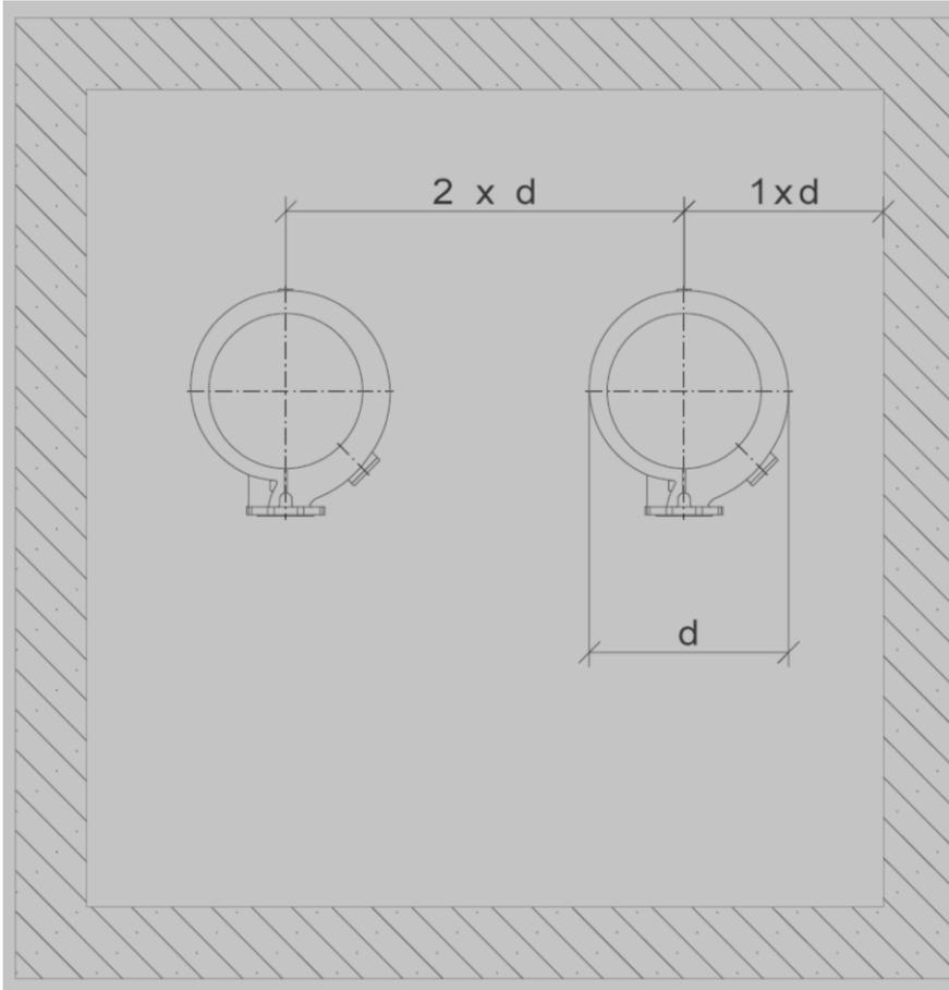
**General spacing for wet pit pumps with both pumps in the control sequence**
