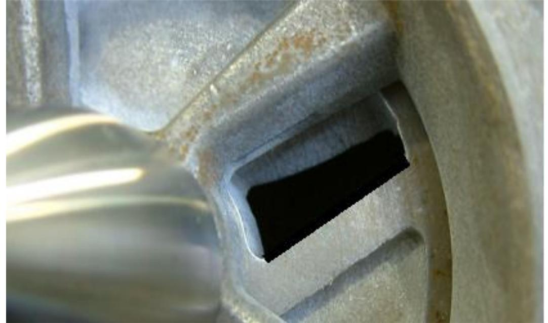
Check tolerances between the cutting surfaces for cutting impellers
