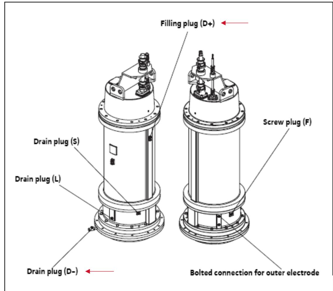
Fig. 7-1: Position of the screw plugs
