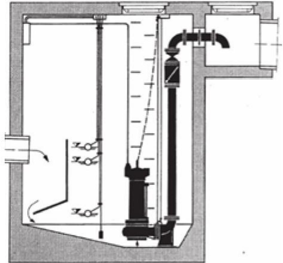
Preferred approach is along the floor at low velocity (1-2 fps) to the pump
