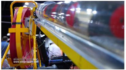
FELL Benchmark Testing of Plastic Pipe (2012) in accordance with ASTM F2550-13 (2018).
