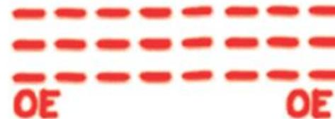
Marks shall be placed at the beginning and the end of the locate and at a minimum interval of two feet but not more than fifty feet throughout the locate as needed to clearly identify the route of the underground utility.
