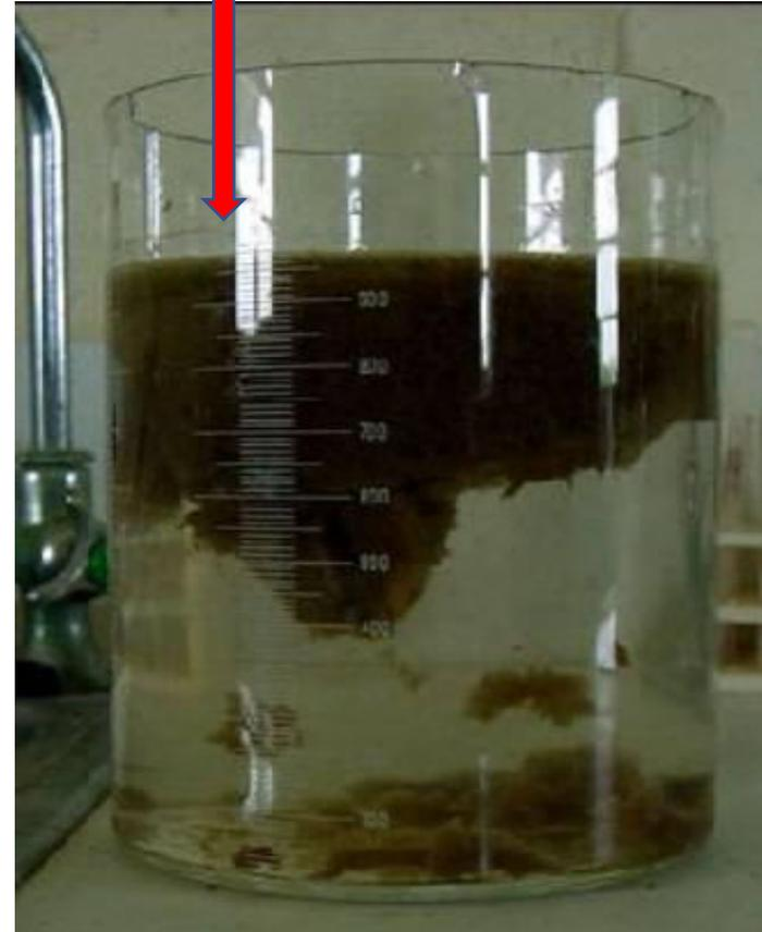
Rising sludge indicates denitrification, look for small nitrogen bubbles on top of clarifier.
