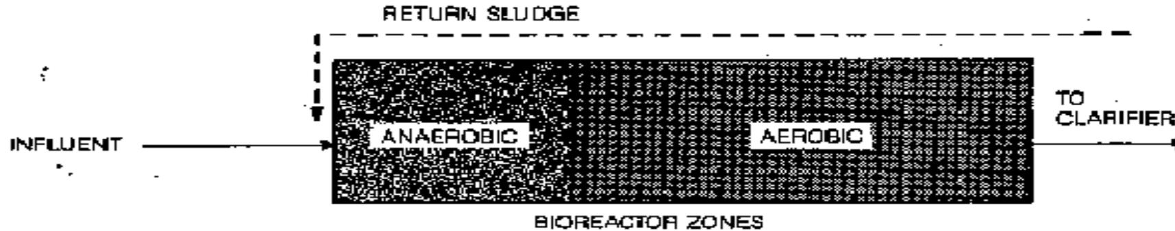
NOTICE: BOD is being reduced while phosphorous is being released in the Anaerobic Zone.
