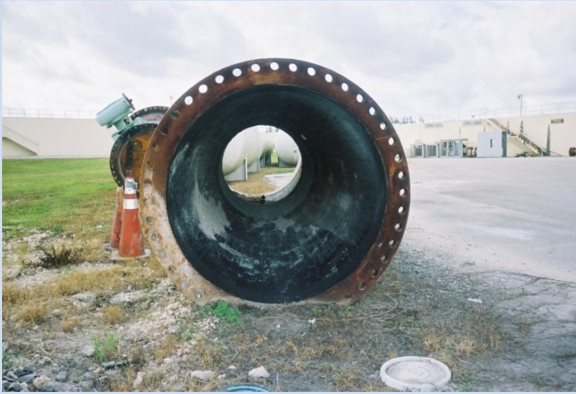
72" Venturi Meter, too big to be tested off sight
