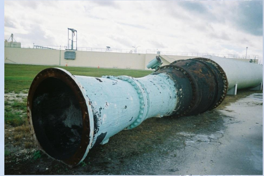
72" Venturi Meter, too big to be tested off sight
