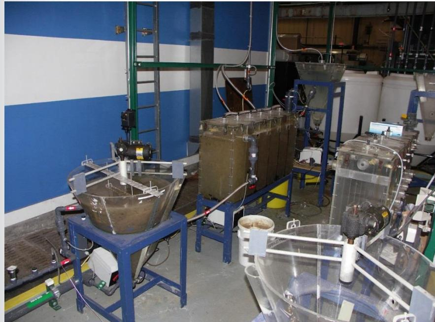
Activated sludge experimental set-up:
