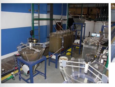
Activated sludge experimental set-up: assessing how contaminants travel through wastewater treatment systems Wastewater test bed: assessing persistence of contaminants on sewer infrastructure
