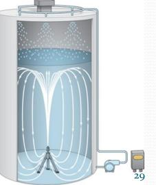
Diffused Aeration – Min 4-Ft headspace Tiny Bubbles Air Bubble Size Air to Water Ratio Depth of Water Above the Diffuser Detention Time Water Temperature Geometry of Tank (Baffling)
