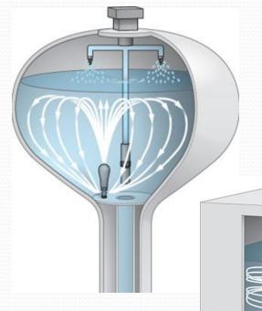
Droplet size Travel Distance Water Temperature Ice Formation, typically spray not operated in Winter
