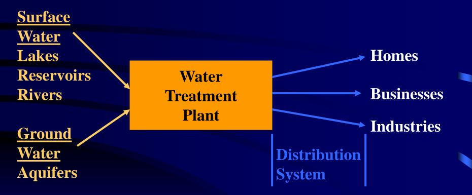
Fresh water is collected from Surface and Ground Water Sources, processed at a Water Treatment Plant to produce drinking water, and is distributed through pipes to the Customers.
