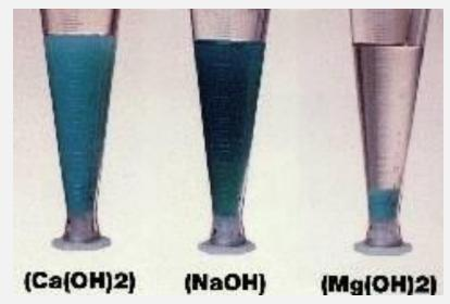
When compared to calcium hydroxide (far left) and sodium hydroxide, magnesium hydroxide (far right) substantially reduces sludge volume as shown in this laboratory acid neutralization test.
