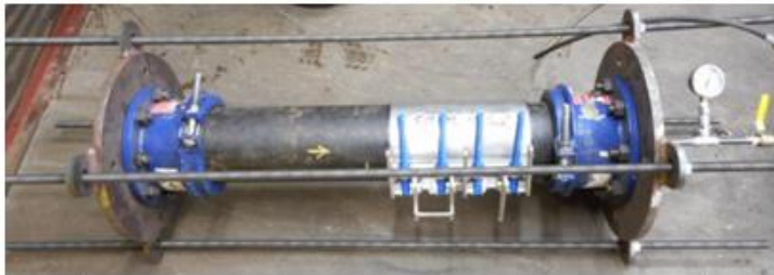
Ductile Iron Pipe Test Fixture with 3/4" Dia Drilled Hole
