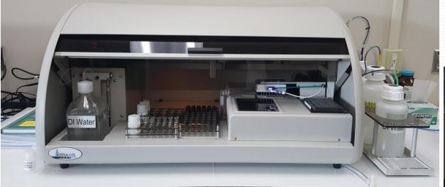
Samples and Standards are loaded onto the Cyanotoxin Automated Assay System (CAAS)
