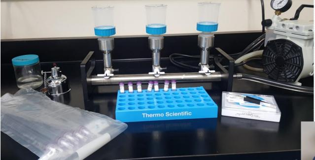
• DNA Extraction begins with a filtration step using sterile equipment
