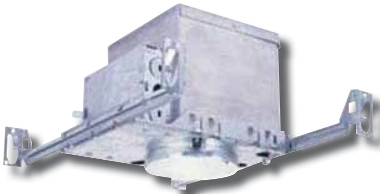
Housing adjusts to accommodate up to 1 1/2" ceiling thickness. 4 1/8" height allows use in 2" x 8" joist construction. Integral T-bar installation slots
