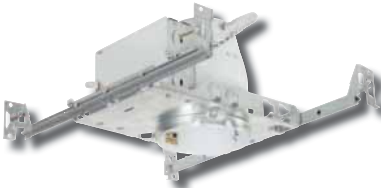
Adjustable hanger bar with 16" - 24" joist span. 4 1/8" height allows use in 2" x 8" joist construction. Integral T-bar installation slots.
