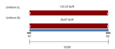
Section: 1200S200-97 (50 ksi) @ 16 in" o.c. Single C Stud (punched) Maxo = Va = 8147.0 lb I = 30.175 in^4 11626.1 ft-lb
