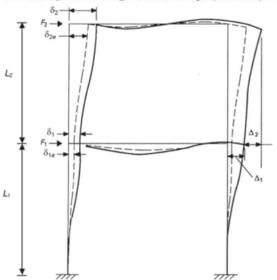
Note:  $\Delta_j = \text{story drift}$ ;  $\Delta_j / L_j = \text{story drift ratio}$ ;  $\delta_g = \text{total displacement}$ ; I = level under consideration.
