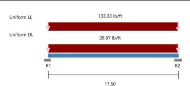
Section: 1200S200-97 (50 ksi) @ 16 in" o.c. Single C Stud (punched) Maxo = 11626.1 ft-lb Va = 8147.0 lb I = 30.175 in^4
