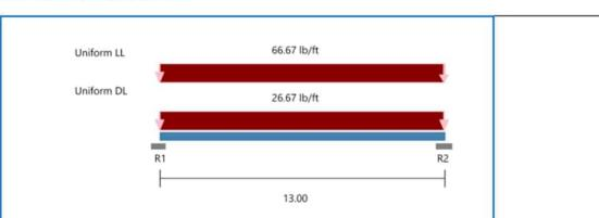
Section: 1200S162-68 (50 ksi) @ 16 in" o.c. Single C Stud (punched)
