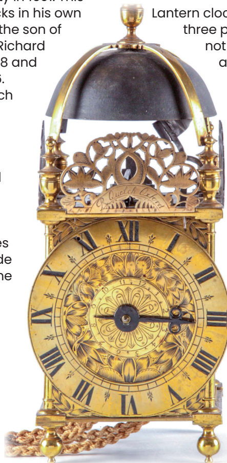
Figure 1. Front view of the Quelch clock, pre-restoration. The dial shows the typical second-period shading of the tulip flowers and the half hour markers. Note the canon pinion and minute-hand shaft for the hands and the unsuitable replacement hand. PHOTO BY GEOFF COX.
