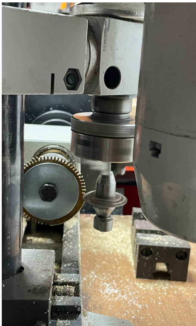
Figure 12. The 64-tooth hour wheel cutting. PHOTO BY GEOFF COX.
