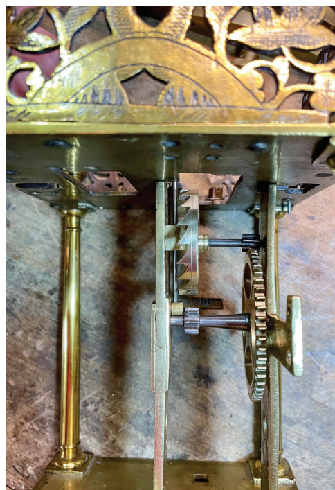
Figure 8. The short bottom verge arbor potence. PHOTO BY GEOFF COX.
