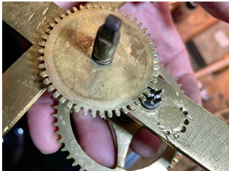
Figure 10. Space constraints of the 48-tooth hour wheel. PHOTO BY GEOFF COX.
