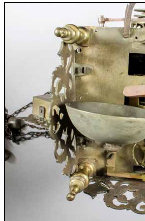
Figure 8 (above). Front fret nudged forward showing empty pin hole (pin top corroded into lug), shortened left lug, normal right lug held by a conventional screw. Photograph by Geoff Cox.
