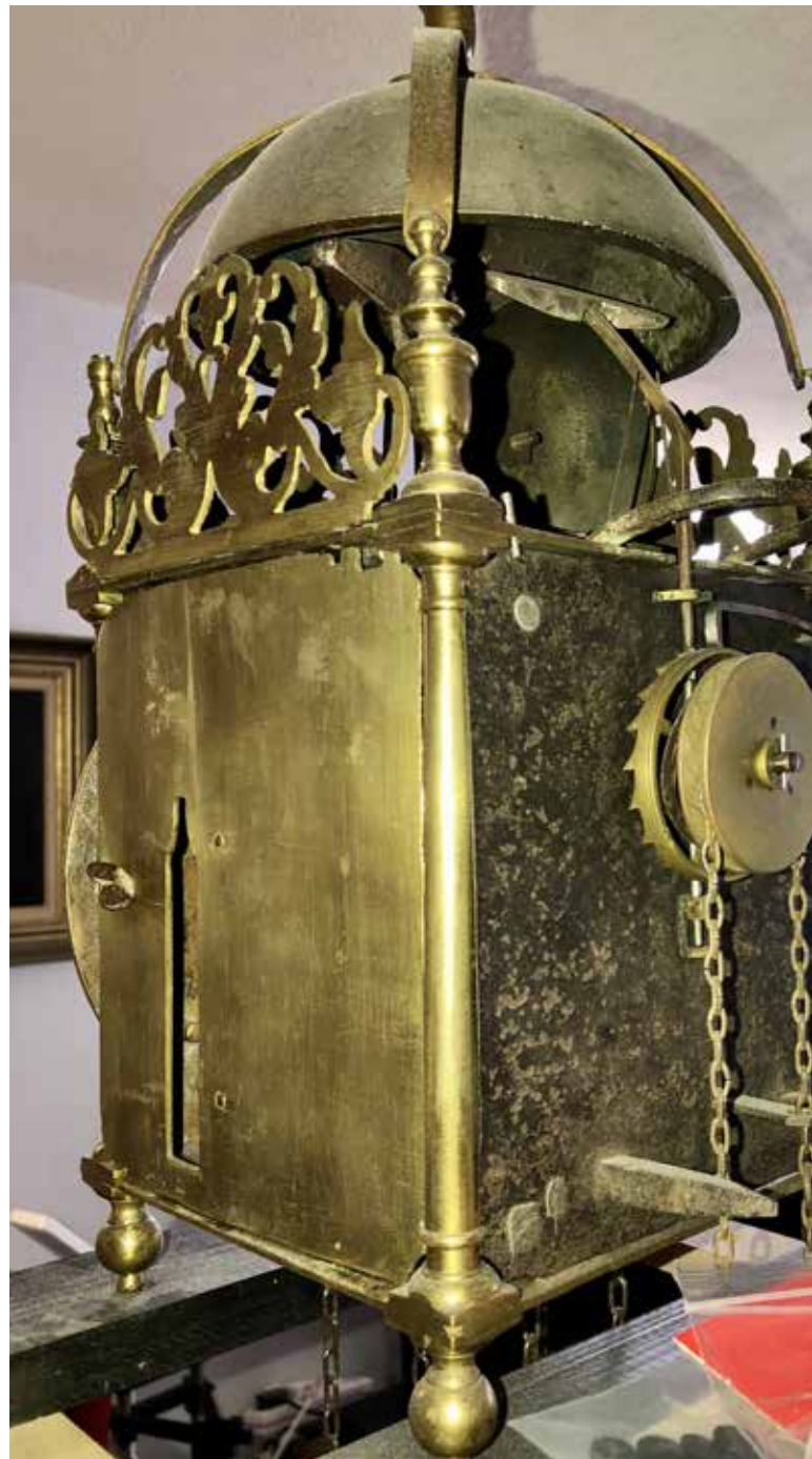
Figure 5 (right). Rear view showing the original alarmwork and the side door with the wing removed, as it was when first made. Photograph by Geoff Cox.
