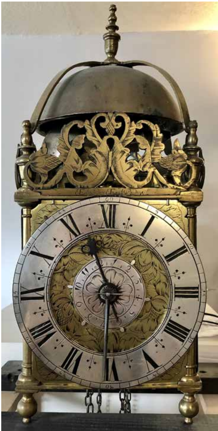
Figure 2 (above). This photograph was taken recently with its wings removed, as it looked when first sold from the East workshops. Probably then driven by rope rather than by a chain. Photograph by Geoff Cox.
