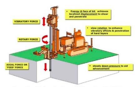
Basic Principle of Sonic Drilling
