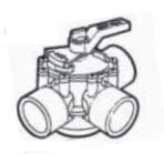
MAIN DRAIN(s) at the bottom of the deep end of the pool. The flow is controlled by 3-way valve at the intake to the pump. Under normal operation both lines should be fully open. If the water in the pool is too low, the pool may be run with the SKIMMER closed and MAIN DRAIN open until the water is returned to normal operating level but it is dangerous to swim with this setting. The MAIN DRAIN is closed for vacuuming.
