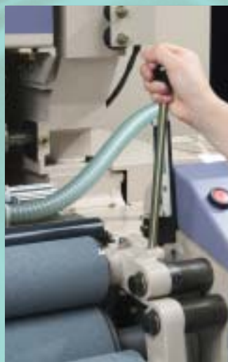
Take-up roll lift up with a simple handle operation
