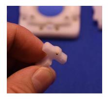
A gold coated spring load contact pin is used to create a trouble free electrical connection to the front of the sample film.
