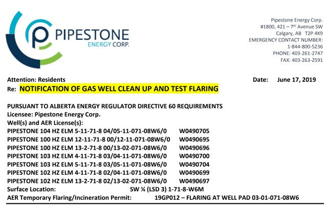
Pursuant to the Alberta Energy Regulator (AER) Directive 60: Upstream Petroleum Industry Flaring, Incinerating and Venting (March 2018), Pipestone Energy Corp. hereby gives notice of sour gas well clean-up and test flaring at the above surface location as shown on the attached Residential Notification Map. All residences within three kilometers of the wellsite are to be given this notification.
