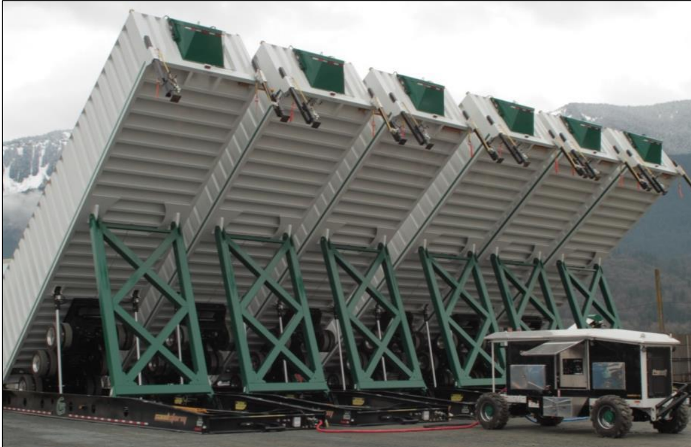
The SandStorm proppant delivery system is a mobile, rapid-deployment proppant handling system that delivers unmatched storage capacity, dust control and digital automation. Calfrac Well Services Photo
