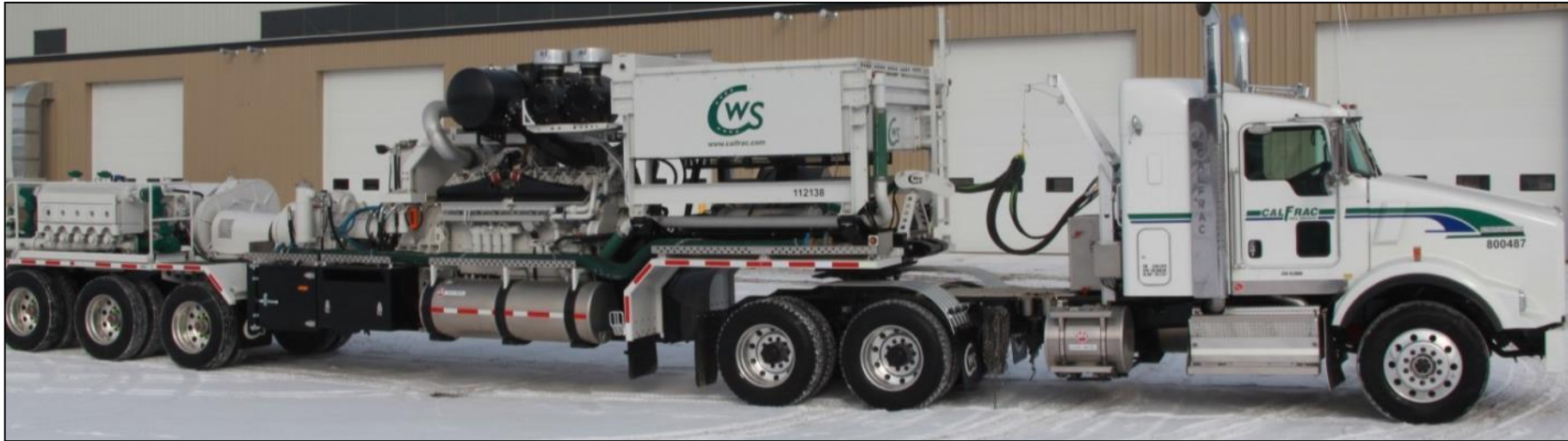
Quintuplex pump delivers maximum power along with dual fuel capability. Calfrac Well Services Photo
