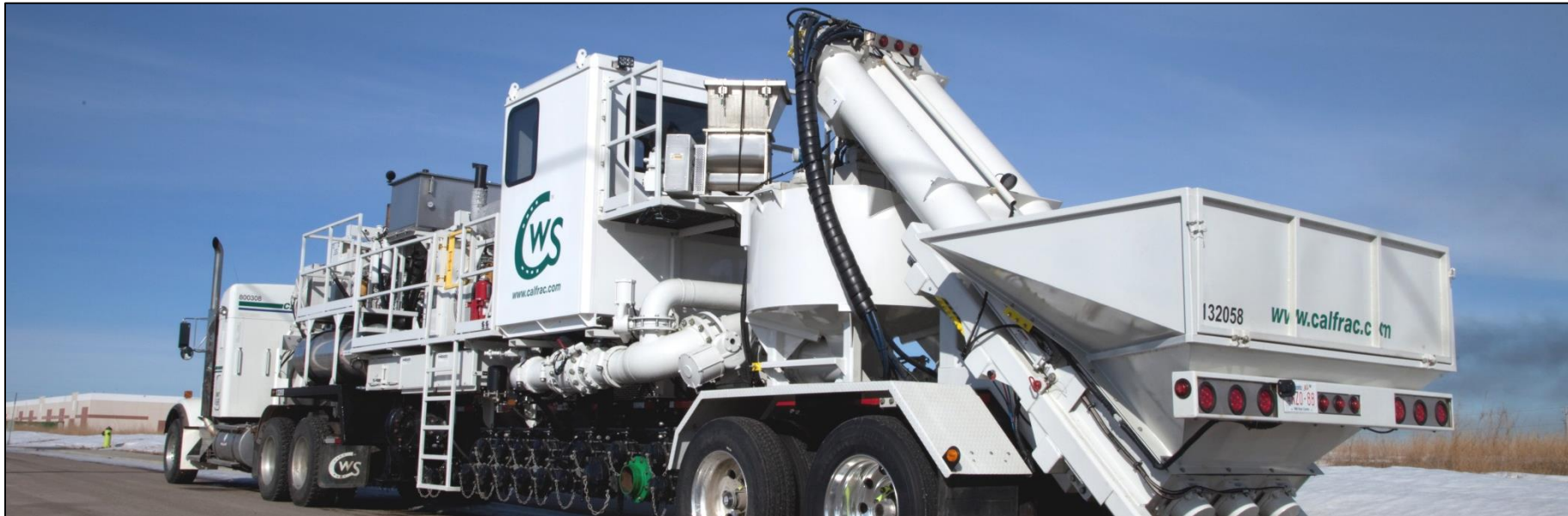
This blender delivers the high pump rate required for unconventional and tight gas reservoirs. Calfrac Well Services Photo
