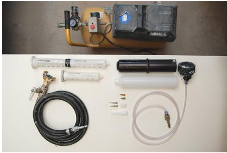
Left - syringes originally used. The clay is extruded with compressed air.
