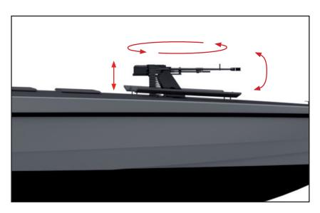
The front machine gun, also with a wide range of rotation, is hidden in its compartment inside the boat and when requested it comes out electrically
