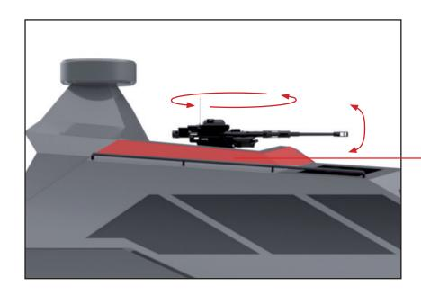
The upper machine gun holds a wide angle of rotation, and is protected by a conveyor that in addition to protecting the base of the weapon, also has an aerodynamic function. In the rear, the support for the radar and the various antennas also takes a shape stealth and aerodynamics.
