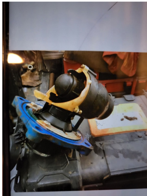
Debris in Turbine for Whitlock Meter was causing meter not to report.
