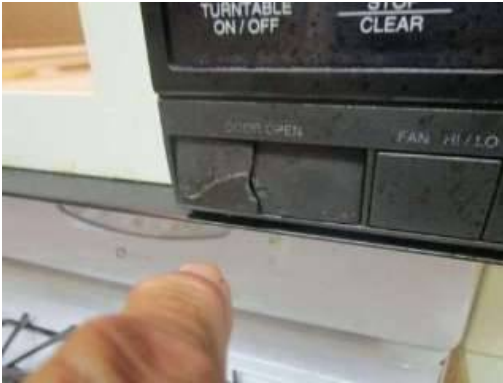
Photo 10-4 The microwave door open button is broken.
