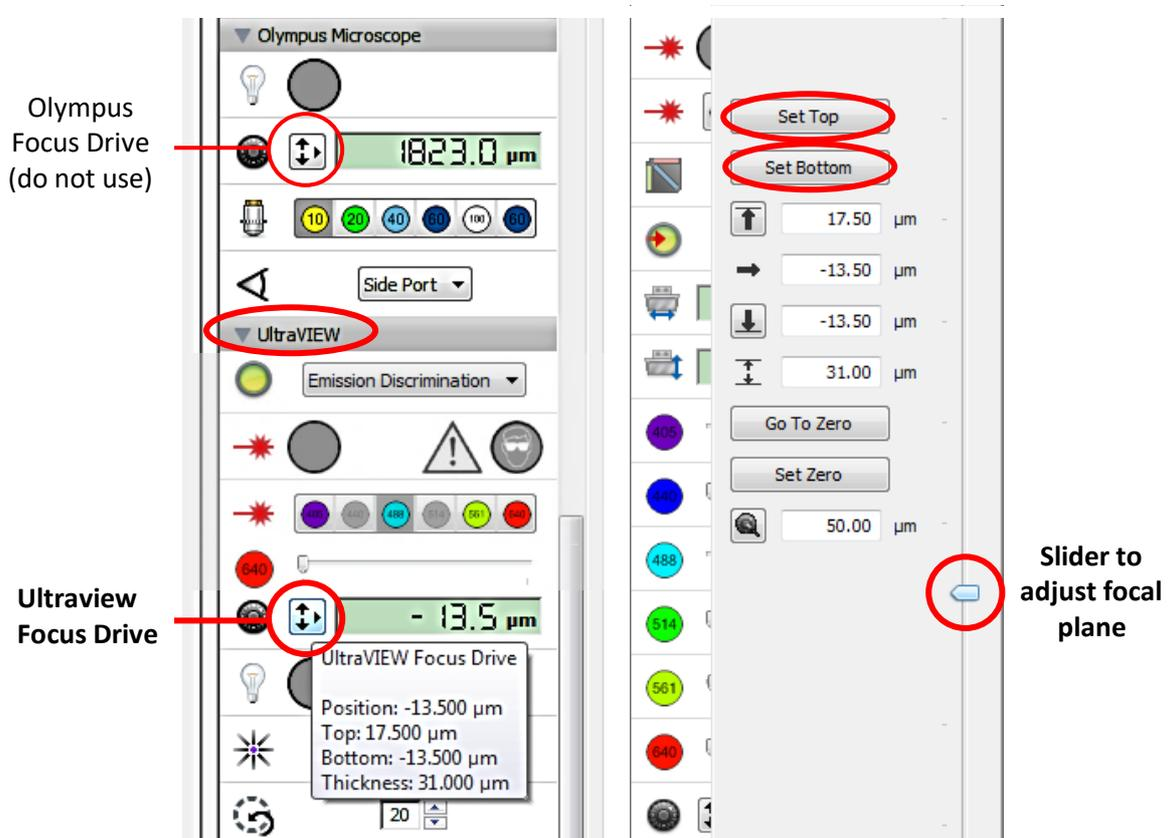
2. Update experiment protocol in **Acquisition setup** to include Z- stack with Ultraview Focus Drive. Start the experiment protocol.
