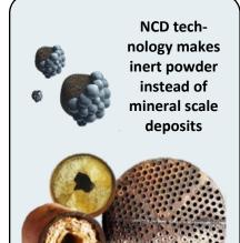
As cooling systems evaporate water during heat-rejection, minerals and salts originating in the makeup water concentrate in the cooling system. Calcium, unlike other minerals and salts, precipitates in a hotter operating environment. Scale deposits reduce efficiency/increase the energy required to provide cooling and, can promote under-deposit corrosion and harbor microorganisms.
