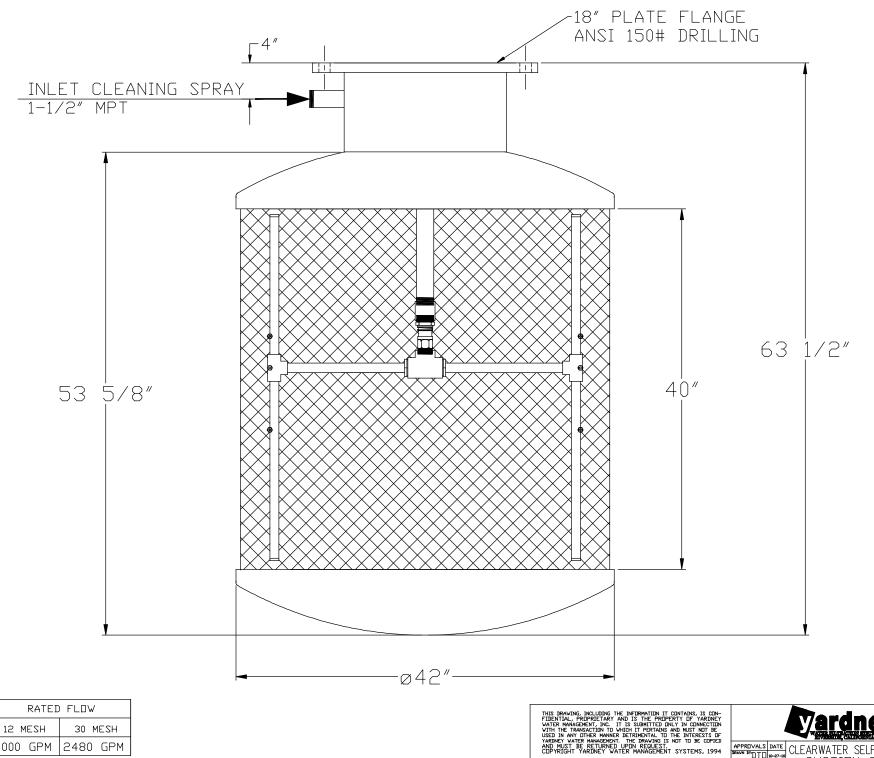
MODEL 12 MESH CW4000 4000 GPM 2480 GPM CLEANING SPRAY FLOW 44 GPM @ 40 PSI MIN, 65 PSI MAX
