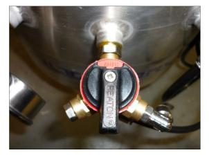
gradually and in stages so that the pressure stays at around the normal operating pressure of the system. Once the system is filled you will then be able to open the valve fully.
