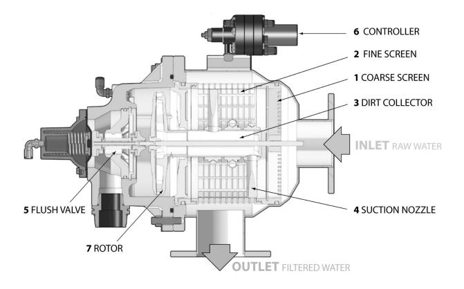
Put simply the Filtaworx filter cleaning cycle works in a similar way to a vacuum cleaner, cleaning the solids off the fine screen with suction nozzles that rotate and spiral up and down to clean the whole fine screen area.
