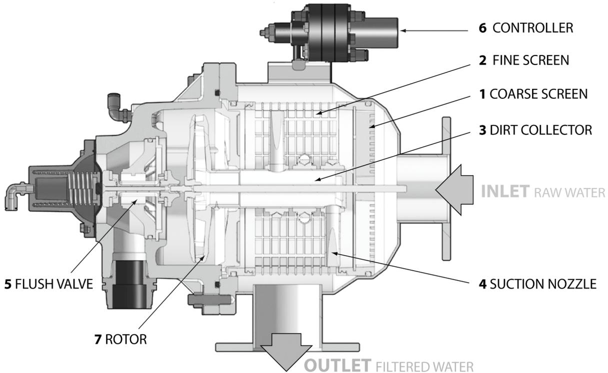
Put simply the Filtaworx filter cleaning cycle works in a similar way to a vacuum cleaner, cleaning the solids off the fine screen with suction nozzles that rotate and spiral up and down to clean the whole fine screen area.
