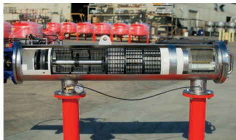
Twist-lock sectional screens provide easy cartridge replacement.
