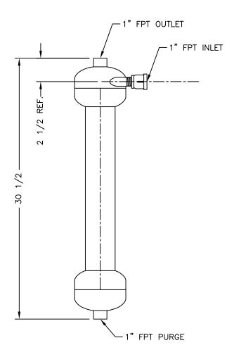
FLOW RATE: 18 - 38 GPM.
