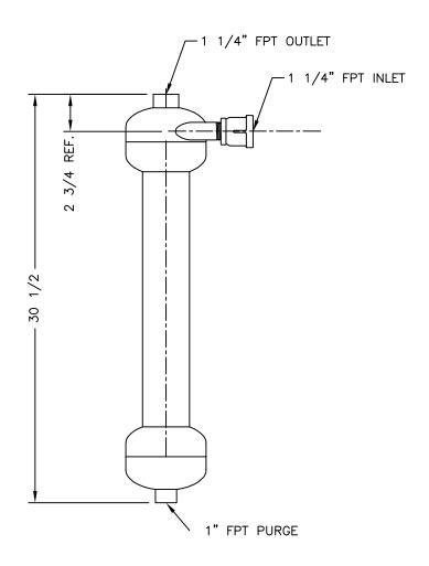
FLOW RATE: 26 - 52 GPM. PRESSURE RATING: 150 PSI. SHIPPING WEIGHT: 26 LBS.
