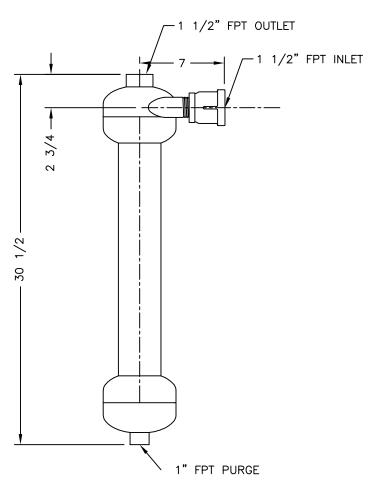
FLOW RATE: 38 - 79 GPM. PRESSURE RATING: 150 PSI. SHIPPING WEIGHT: 26 LBS.
