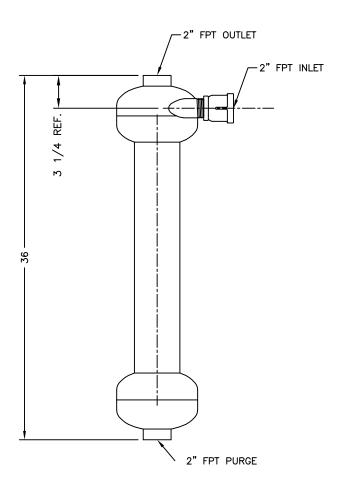
FLOW RATE: 63 - 120 GPM. PRESSURE RATING: 150 PSI. SHIPPING WEIGHT: 44 LBS.
