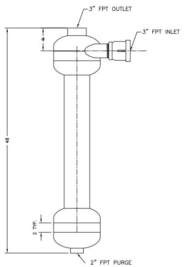
FLOW RATE: 125 - 260 GPM. PRESSURE RATING: 150 PSI. SHIPPING WEIGHT: 75 LBS.
