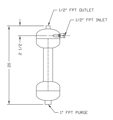
FLOW RATE: 4 - 10 GPM, PRESSURE RATING: 150 PSI, SHIPPING WEIGHT: 13LBS,
