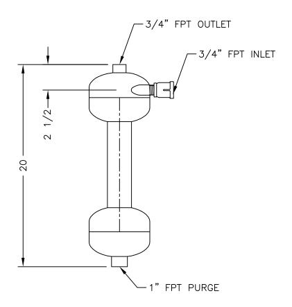
FLOW RATE: 10 - 20 GPM.
