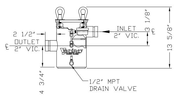
MAX PRESSURE MAX FLOW MODEL **GPM** PSI SB 5 110 150
