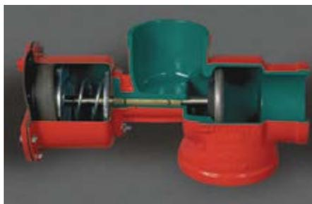
Our patented cast-iron backwash valve has the lowest pressure drop in the industry and is designed to be 100% field serviceable with basic hand tools. Valves feature non-corrosive stainless steel shafts, brass bushing, durable molded polyurethane seals, fusion epoxy lining, and a grease fitting for valve shaft lubrication.
