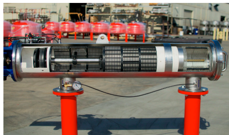
Twist-lock sectional screens provide easy cartridge replacement.
