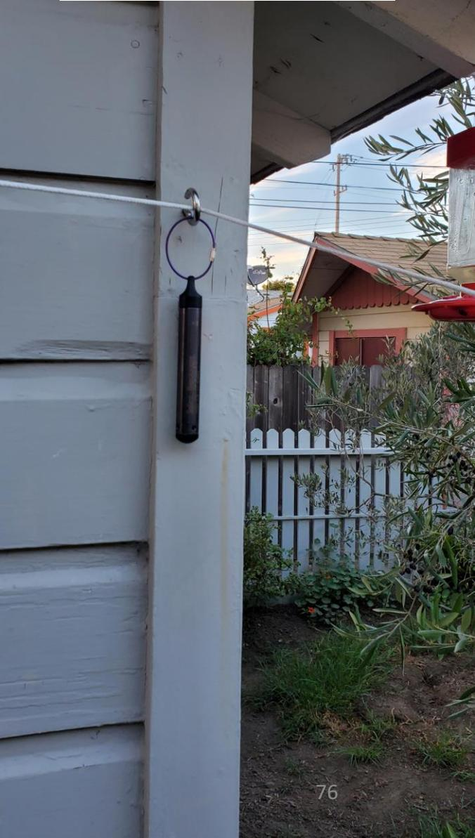
10/15/22: repair AVW1; 20 ft (6-in diameter) well, about 7 ft static water level
