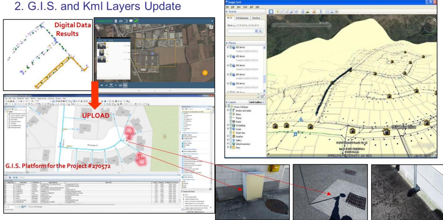
The final results of the survey and post processing activities is a G.I.S. available on-line and interactive, with editable features and position such us manholes, cabinets and water connections.
