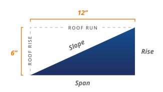
**ROOF PITCH = RISE / SPAN**
