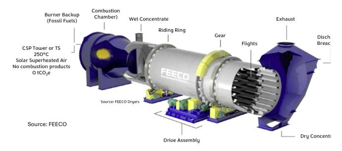
Dryers are commonly used for drying ore concentrates such as copper, spodumene, zinc, gold, lead, silver, nickel, cobalt and manganese or drying iron ore pellets.
