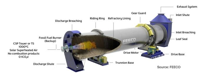
A rotary kiln (calciner) is a rotating heat treatment furnace used for continuously calcining or sintering materials to cause a chemical reaction or physical change. This technology is utilized by the Mining Industry for the calcination (lime, etc), reduction roasting and sintering/hardening for ores and other materials.
