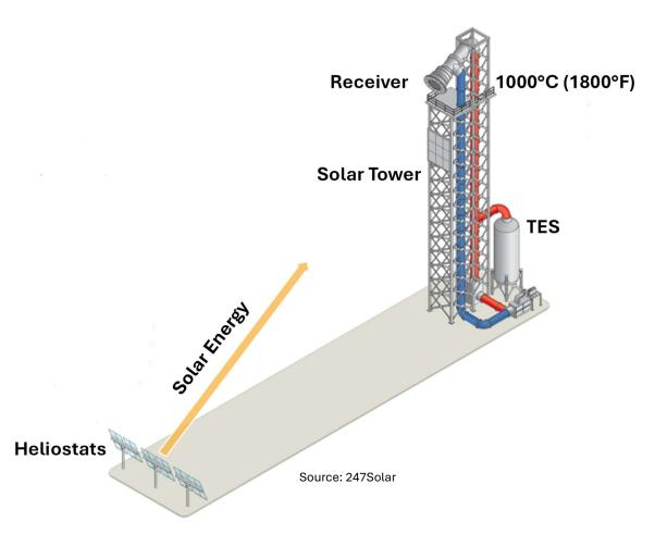
**Solar towers** (power towers) use many sun-tracking mirrors called heliostats to focus sunlight onto a receiver at the top of a 35m tower. The superheated air (**1000°C**) produced from this renewable energy strategy can be **utilized** and **stored** (ceramic pellets) to provide medium and high temperature process heat for the previously discussed mining processes, thus eliminating or reducing fossil fuel usage.
