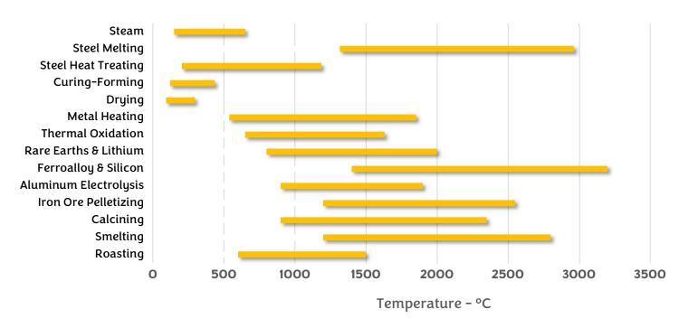
Steam production and Dryers are a good example of a Medium Temperature (**250°C - 600°C**) mining process. For example, Dryers are common in such operations as drying ore, concentrates (copper, zinc, lead, gold, silver, PGM, lithium, nickel, cobalt and manganese) and iron ore pellets.
